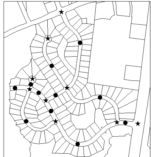
A graphic from the Town of Cary, NC Code that illustrates a connectivity index of 1.2 (links are shown as circles and nodes are shown as stars). The illustration has 11 links and 9 nodes for an index of 11 / 9 = 1.2
